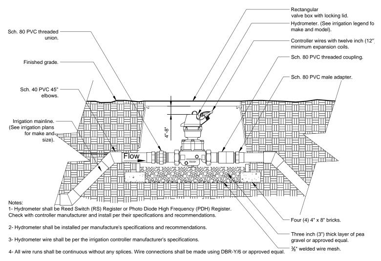
5- Valve box shall be wrapped with a minimum 3 mil. thick plastic and secure it to the valve box using duct tape or electrical tape.
